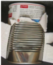
Dented without sharp edges or creases and not over seam
