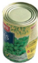
Dented without sharp edges or creases and not over seam
